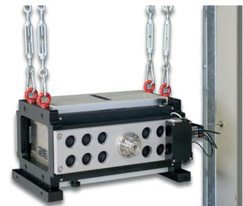
APS 420 with modal stinger (APS 8610) and steel cable kit (APS 8612) prepared for free body mode operation
